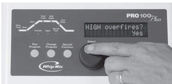
Rotate Knob to “Cal – High Fusing”, Press Next The furnace would display “High Fusing – Overfires?” on the top line and Yes or No on the second line.
