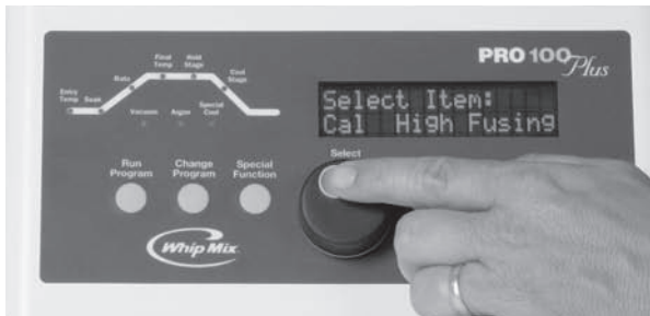
Rotate Knob to “Cal – High Fusing”, Press Next The furnace would display “High Fusing – Overfires?” on the top line and Yes or No on the second line.
